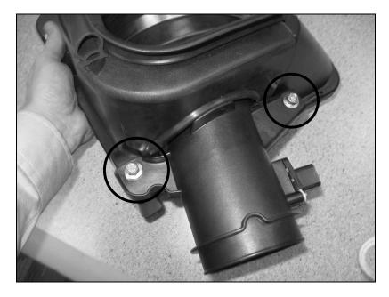
14. Orient the filter so it sits at a slight angle forward as shown.
