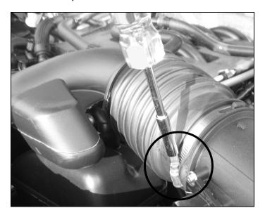
4. Loosen the hose clamp that connects the clean air tube to the throttle body.
