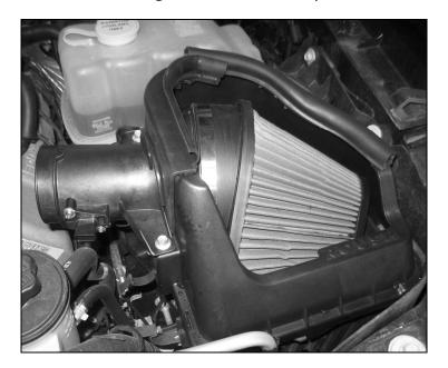
16. Install the new clean air tube between the throttle body and the new ROUSH air box lid assembly. Secure the clamps for the air box lid and tighten both clamps on either end of the clean air tube.
