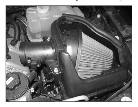
15. Install the new ROUSH clean air tube between the intake and the new ROUSH air box lid assembly. Secure the clamps for the air box lid and tighten both clamps on either end of the clean air tube.
