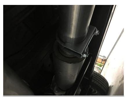
• Install the hanger clamp onto the mid-pipe and into the factory rubber isolator
