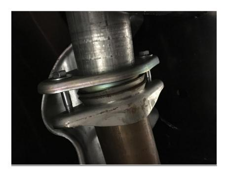
Install the mid-pipe that is the appropriate length that was previously determined using a 3" clamp
