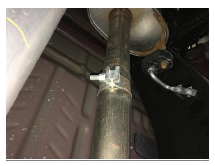
• Loosen the factory mid-pipe flange bolts
