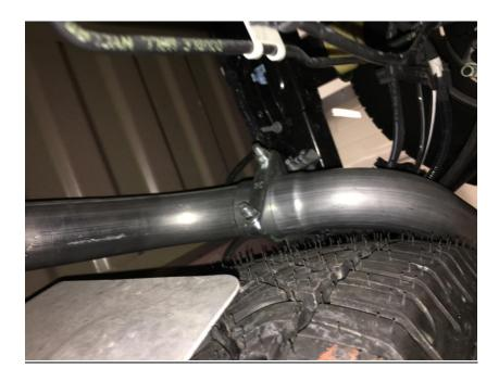
• Install the passenger-side over axle pipe into the lower muffler outlet
