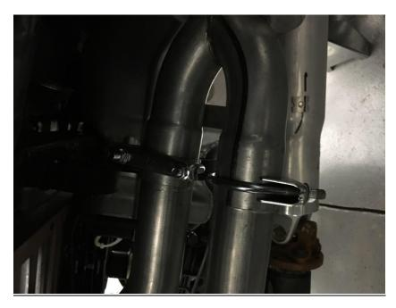
• Install the driver-side over axle pipe into the left upper muffler outlet
