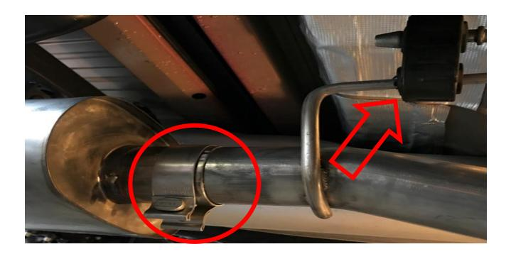
**4.** Slide - 2'' clamp onto each exhaust tip and slide over muffler section and place in hanger and tighten the 2 - 15mm nuts
