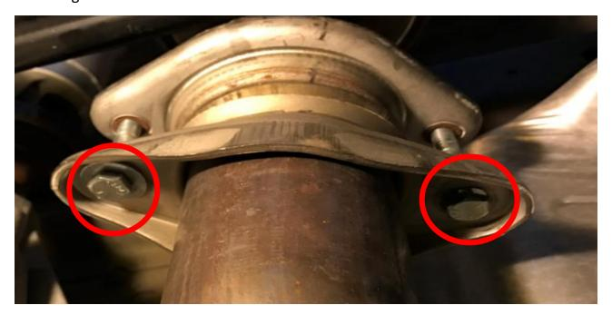
2. Loosen the resonator nut with the 15mm socket on the 3" clamp
