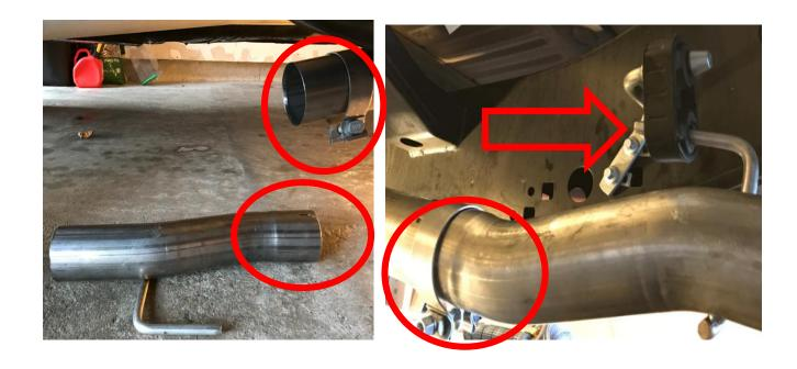
**3.** Slide a 3" clamp on the resonator extension pipe and slide muffler over pipe and into the rubber factory hanger, loosely tighten 15mm nut
