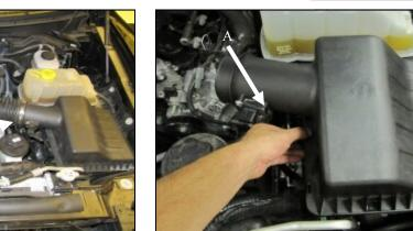
2. A.) Disconnect the Mass Air Flow (MAF) Sensor.
