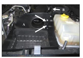
**8. A.)** Mount the Intake Tube to the Rear Panel using the two 1/4-20 Button Head Bolts (#11) and 1/4" Flat washers (#12).
