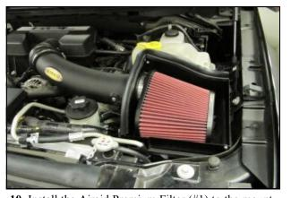
10. Install the Airaid Premium Filter (#1) to the mounting flange inside the quick fit assembly. For **SVT Raptor** vehicles: Complete the installation by attaching the Short Weather Strip (#6a) to the top of the panels as shown.
