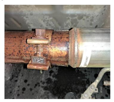
Make sure the exhaust clamp that was supplied with the kit is installed prior to sliding the over the axle pipe onto the muffler. Take a second to apply the supplied anti-seize to the threads of the new clamp. Make sure the muffler is rotated so the front hanger aligns with the grommet on the truck. Once the over the axle pipe is installed onto the muffler, using a 15mm deep socket, tighten the clamp. Now tighten the clamp on the front of the muffler using a 15mm deep socket. Torque: 45Ft lbs.
