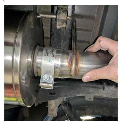
Install the grommet onto the muffler hanger. Spray with soapy water first to make it slip on easier.
