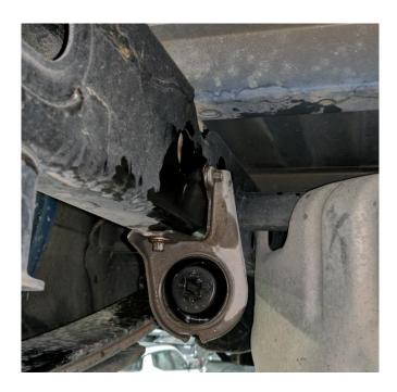
Install the middle grommet bracket onto the over the axle hanger. Install the grommet bracket by using a 10mm deep socket. Make sure the side without a bolt gets slid back into the slot in the frame.
