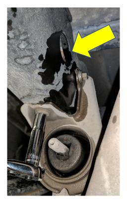
In order to remove the exhaust from the truck, you must twist the whole system towards the driver's side of the truck (counter clockwise), or if someone is helping, twist the tail pipe up, and then pull back. The OEM exhaust has a notch in the pipe that has to be cleared. Once the pipe is removed, work the exhaust over the axel, towards the front of the truck.
