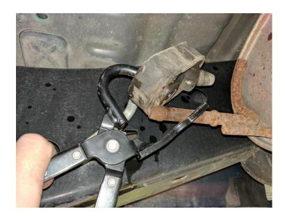
Using a 10mm deep socket, remove the bolts holding on the grommet bracket at the top rear of the muffler. Once you remove the bolt, you will have to slide the bracket towards the driver's side of the truck to separate it from the truck.
