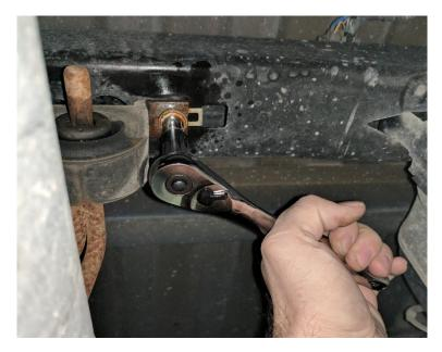
Remove the last grommet bracket by using a 10mm socket. At this point, the exhaust is only being held up where it connects to the cat. \*by using the access hole in the frame, you can spray the top of the bolts with penetrating oil to help with removal – See Arrow\*
