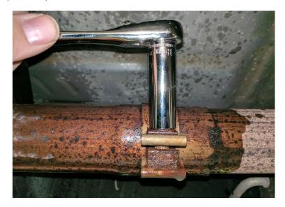
Spray rubber grommets with soapy water prior to removal to help the hangers slide out. Use exhaust grommet removal tool to remove the grommet at the front of the stock muffler. If you do not have access to a grommet removal tool, you can use a screw driver to work the grommet off by sliding it next to the hanger and pulling down.
