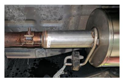
Slide the exhaust clamp onto the exhaust tips. Apply supplied anti-seize to the threads of the bolt prior to tightening. Align the exhaust tips with the bed of the truck. Once they are in the desired position, tighten the bolt using a 15mm deep socket. Torque: 45 Ft lbs.
