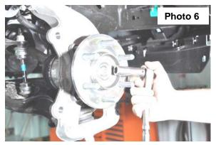
9. Using a 21mm wrench and a 1 1/16" socket loosen the lower control arm bolts. Do not remove the bolts just loosen them so you can later swing the lower control arm down.
