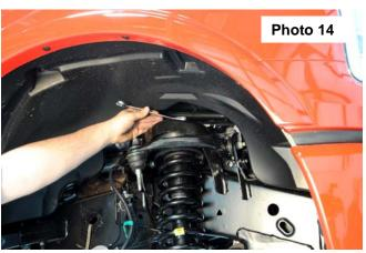
20. Install the factory studs back into the barpin on the lower mount of the strut. It may be necessary to hit the top of the strut with a hammer to seat the splines before tightening the factory nuts with a 18mm. **See Photo 15.**
