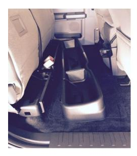
4) Loop safety straps around seat bracket cross bars and through the slots in the wall of the Gear Box (see Figure 3).
