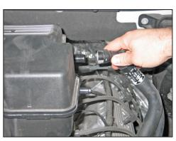
7. Release the locking tab and then disconnect the crankcase vent hose from the intake plenum.
