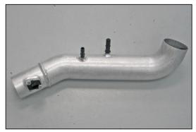
30. Install the  $\frac{1}{2}$ " hose fitting into the K&N® intake tube as shown.
