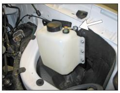
16. Secure the coolant bottle assembly to the inner fender using the provided hardware and spacer.
