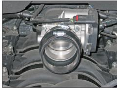
25. Install the provided silicone hose (084057) onto the throttle body and secure with provided hose clamp.
