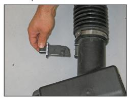
27. Remove the two screws securing the mass air sensor into the upper air box housing, then remove the mass air sensor from the housing.
