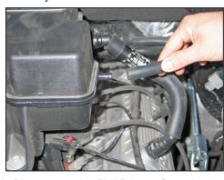
6. Disconnect the EVAP hose from the intake plenum.
