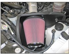
34. Mount the K&N® air filter onto the filter adapter and secure with a provided hose clamp. Transfer the coolant from the factory reservoir into the K&N® coolant reservoir.
