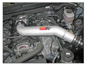
31. Install the K&N® intake tube into the silicone hose attached to the filter adapter. Insert the intake tube's opposite end into the silicone hose on the throttle body, secure each end with the provided hose clamps.
