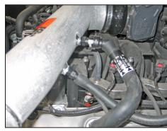
32. Connect the crankcase vent hose to the quick disconnect fitting. Attach the EVAP hose to the  $\frac{1}{2}$ " hose barb.
