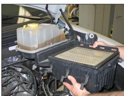
14. Remove the lower air box/coolant reservoir assembly from the vehicle.
