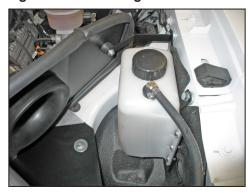
24. Route the coolant reservoir transfer hose to the coolant reservoir. Trim the hose for proper fit, then attach the hose onto the fitting and secure with the provided hose clamp.
