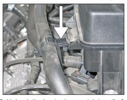
8. Unhook the heater hose retaining clip from the intake plenum.
