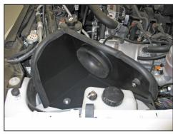
23. Install the heat shield assembly into the vehicle so the inserts align with the air box mounting grommet locations. Secure the heat shield mounting bracket to the inner fender with the coolant reservoir and spacer provided. Then secure the bottom of the heat shield to the inner fender brace with the inserted nuts.
