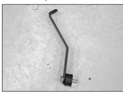
18. Install the provided rubber mounted stud onto the heat shield mounting bracket (083143) using the provided hardware.
