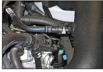
23. Connect the crankcase vent hose to the quick disconnect fitting in the K&N® intake tube.
