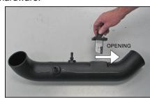
21. Install the mass air sensor assembly into the K&N<sup>®</sup> intake tube and secure with the provided hardware.
