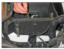
12. Remove the center airbox retaining clip.
