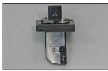
20. Install the mass air sensor into the K&N® sensor adapter as shown. Secure with the provided hardware.
