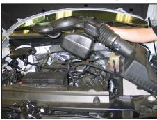
6. Release the three clips securing the upper airbox housing to the lower housing and then remove the intake tube/upper airbox and air filter from the vehicle.
