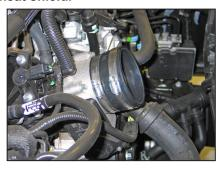
14. Install the provided silicone hose (08630) onto the throttle body and secure with the provided hose clamp.
