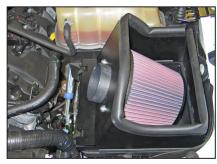
13. Install the heat shield/filter assembly onto the lower airbox and secure with the factory airbox retaining clips.
