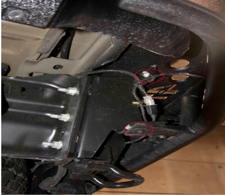
Revolver Rear bumper bolted up using the 3 factory tabs
