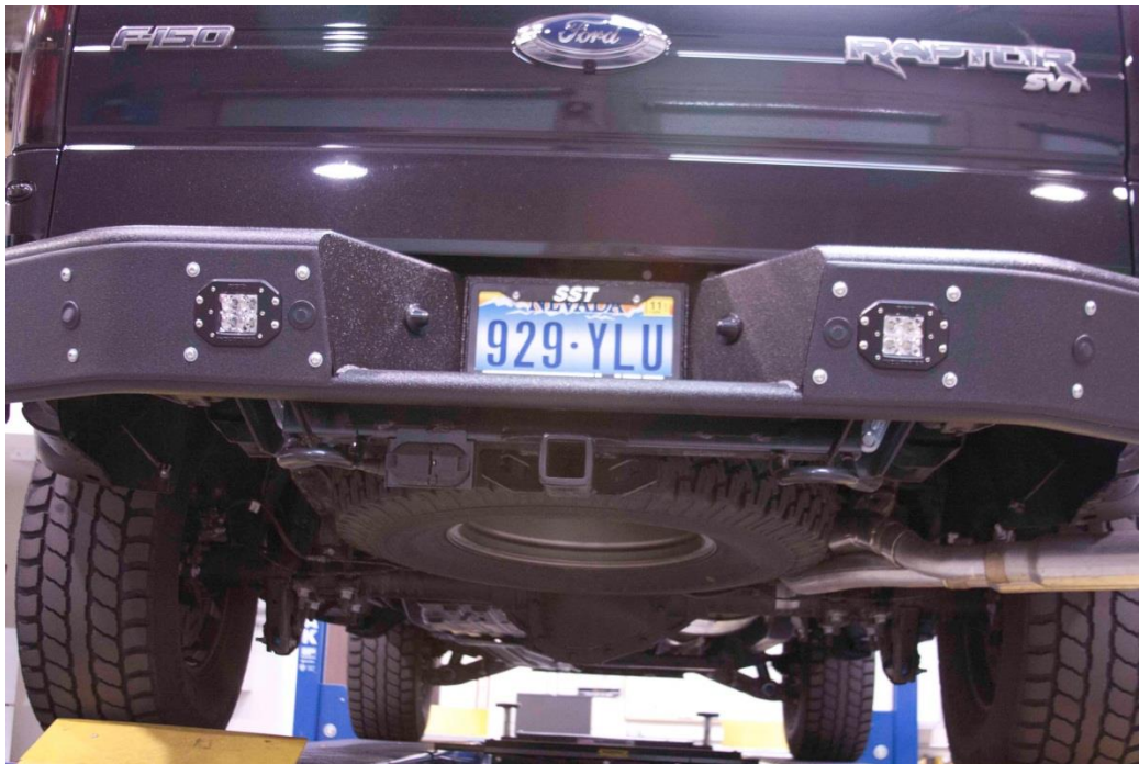
Rear View with bumper and Rigid flush mounts installed rear bumper Install
