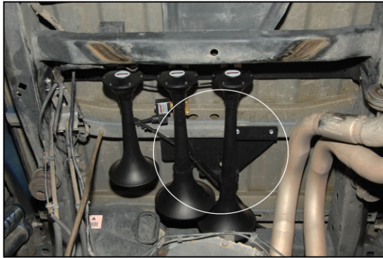
Location of VELO-730 Support Bracket & Mounting Points
