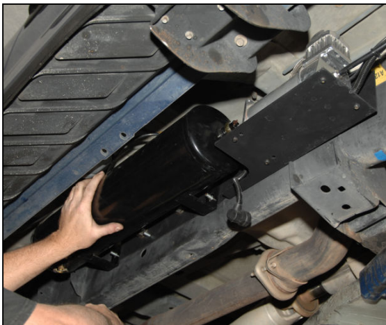
Image C - Air Tank Location on Frame
