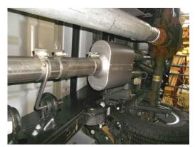
3) Slide the inlet hanger #490HA over the back of the inlet pipe and insert the hanger into the factory rubber mount. Do not tighten this clamp yet. If required, place the extension pipe #26277S onto the back of the inlet pipe. Then place the inlet of the muffler onto the back of inlet pipe and support with a stand. Level the muffler and tighten the clamp at the inlet enough to hold, but still allow for adjustment.
