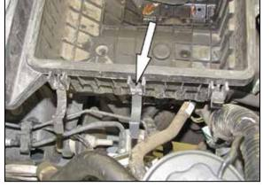
16. Remove the center upper air box retaining clip.
