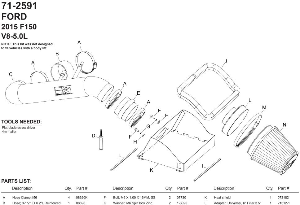
Е Hose; 3-1/2"ID X 2-1/2" L Hump 08699 Edge Trim (39") 102496 1 J 1 NOTE: FAILURE TO FOLLOW INSTALLATION INSTRUCTIONS AND NOT USING THE PROVIDED HARDWARE MAY DAMAGE THE INTAKE TUBE, THROTTLE BODY AND ENGINE.
