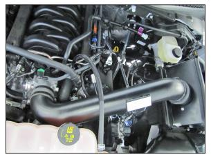
14. Install the K&N<sup>®</sup> intake into the coupling hose at the filter adapter and then into the hose at the throttle body, adjust the tube for best fit and then secure with the provided hose clamps.
