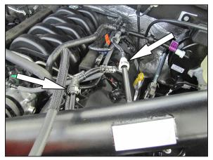
15. Connect the factory EVAP and Crank case vent
