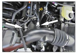
2. Disconnect the EVAP vent connection and crank case vent connection.
