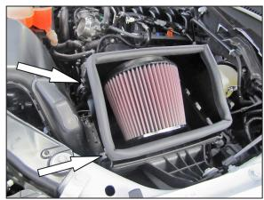
11. Install the filter/heat shield assembly onto the lower air filter housing and secure with the factory retaining clips.
