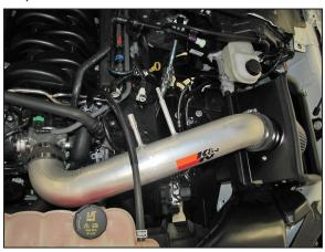
14. Install the K&N<sup>®</sup> intake into the coupling hose at the filter adapter and then into the hose at the throttle body, adjust the tube for best fit and then secure with the provided hose clamps.
