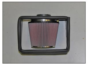
10. Install the air filter onto the filter adapter and secure with the provided hose clamp.
