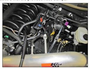
15. Connect the factory EVAP and Crank case vent lines to the fittings on the K&N® intake tube.
