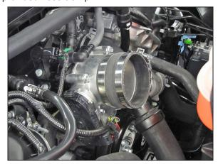
13. Install the provided coupling hose (08698) onto the throttle body and secure with the provided hose clamp.
