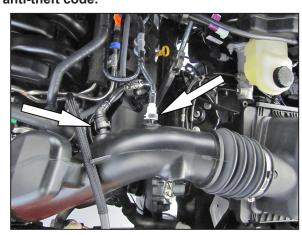
2. Disconnect the EVAP vent connection and crank case vent connection.
