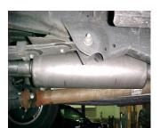
INSTALL MUFFLER # B ONTO HEADPIPE 1  $\frac{1}{2}$ " TO 2". USE CLAMP # F TO SECURE MUFFLER TO HEADPIPE. DO NOT TIGHTEN. USE A JACK STAND TO HOLD UP THE MUFFLER. OUTLETS SHOULD BE LEVEL.
