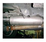
INSTALL MUFFLER # B ONTO HEADPIPE 1 ½" TO 2". USE CLAMP # F TO SECURE MUFFLER TO HEADPIPE. DO NOT TIGHTEN. USE A JACK STAND TO HOLD UP THE MUFFLER. OUTLETS SHOULD BE LEVEL.
