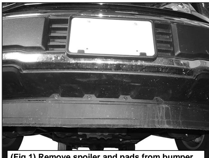
(Fig 1) Remove spoiler and pads from bumper
