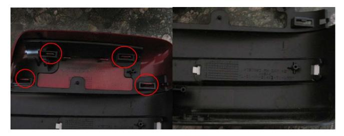
6. Now you can remove the reflector from the housing. Using a flat head screwdriver, gently pry the tab on the outside curved part of the reflector. NOTE: The driver mirror reflector tab on the door side is a fork shape instead of one solid tab.
