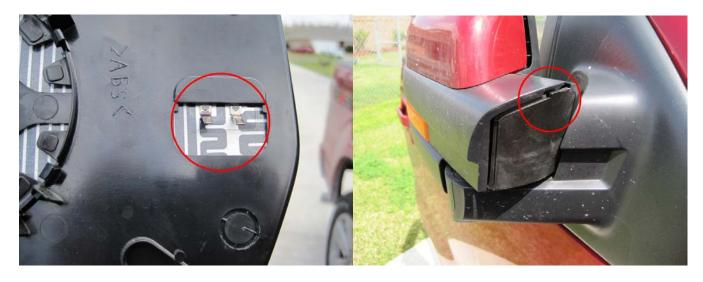
4. Now fold the mirror in towards the door of the truck so you can remove the front half of the housing. Start at the door side of the mirror and pry up as shown. Once you have this part up the housing should pop right off.
