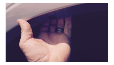
6. Tuck the remaining portion of the Wheel Well Guard behind the fender lip all the way around the fender well opening.
