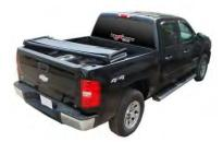
2. PLACE YOUR TONNEAU COVER ON YOUR TRUCK BED WITH THE SAFTEY STRAP CLASPS (STITCHED ON REAR OF TONNEAU COVER) TOWARDS THE BACK WINDOW OF YOUR PICUP TRUCK.
