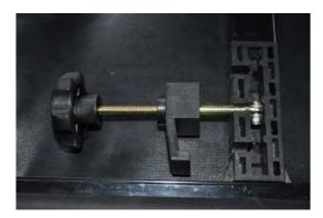
2. HOLD THE CLAMP SO THAT IT IS AGAINST THE TRUCK BED RAIL LIP AND TURN THE ADJUSTMENT KNOB CLOCKWISE UNTILL THE TONNEAU'S METAL CLAMP IS SNUG AND THE COVERS SIDE "Q" SEAL'S ARE COMPRESSED, THEREFORE MAKING YOUR TRUXMART TRI FOLD WATER TIGHT.
