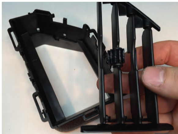
Step 7 Remove the vertical assembly from the vent housing.
