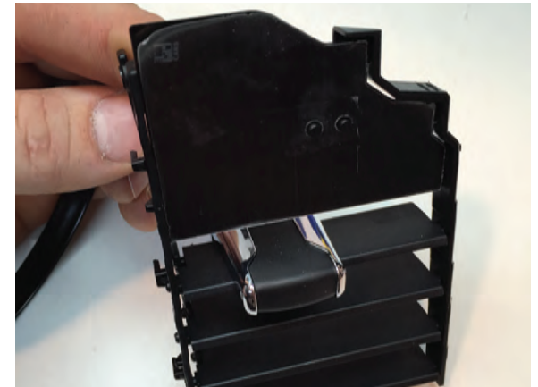
Step 6 Insert display into the vent slat assembly.
