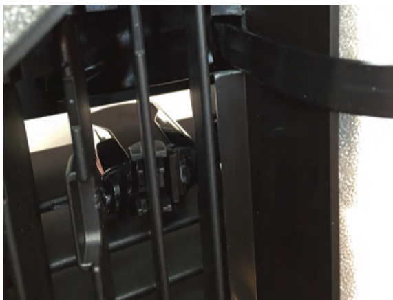
Step 11 Be sure the display cable is flat against the vent housing so it will not interfere with the vertical slats.
