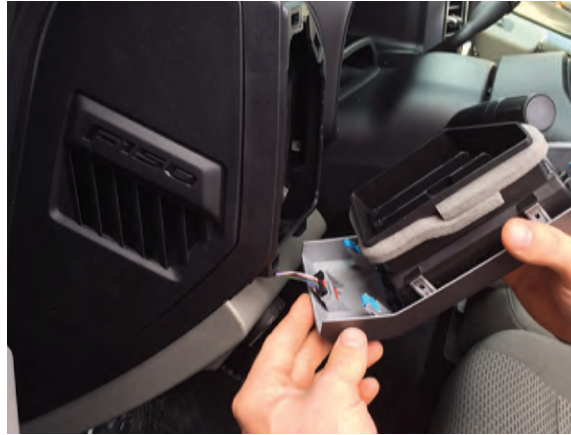
Step 2 Disconnect the connector at the bottom of the vent housing.
