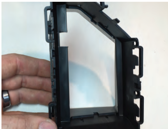
Step 8 Measure down 1" from the top of the vent housing and cut a 7/16" slot as shown in the picture.
