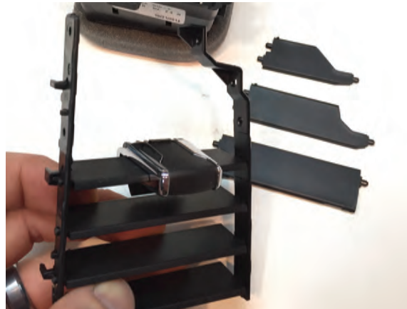
Step 5 Remove the top 3 horizontal slats from the vent slat assembly.
