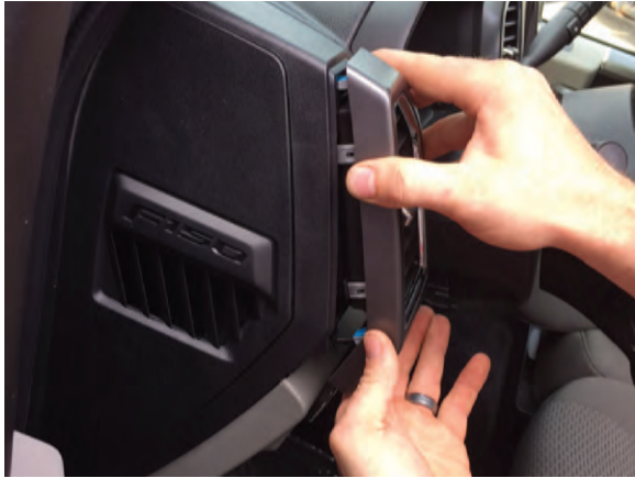
Step 1 Remove vent housing by pulling straight out with a slight upward motion.
