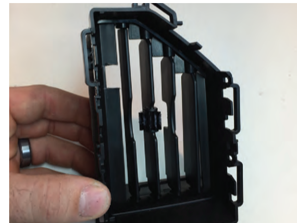
Step 9 Reinstall vertical slat assembly into vent housing.
