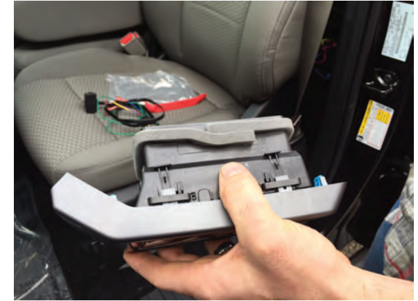
Step 3 Next remove the vent fascia trim by releasing the clips on the side of the vent housing.
