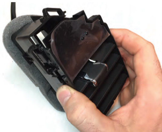
Step 10 With the horizontal slider all the way to the left and vertical slats all the way open, reinstall the slat assembly with display. Feed the display wire through the slot cut in step 5.
