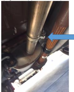
Step 3: Rotate the resonator pipe to unlock the pipe from the muffler and pull towards the front of the vehicle to remove. This was easier when removing the exhaust hanger located before the factory muffler on the passenger side frame to provide more room to work.
