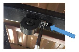
Step 9: Install the Roush muffler into the over axle pipe. The flanged side of the muffler will be facing the front of the vehicle. Slide a supplied 3in exhaust clamp in place over flanged end of the muffler.
