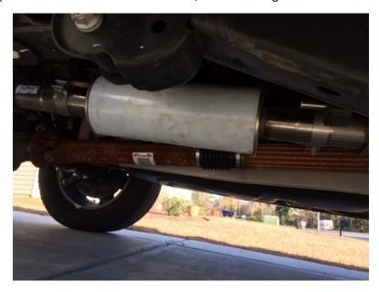
Step 11: Slide the supplied exhaust hanger over the y-pipe for the dual exhaust tips. Slide a supplied 3in exhaust clamp in place over the larger end where it mates to the over axle pipe. Install the larger end on the over axle pipe and then position the hanger so that the open end (looks like a fork) slides onto the rear leaf spring bolt you loosened earlier between the nut and the leaf mount.
