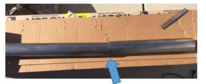
Cut to length using the chart above. My truck was a 145' wheelbase, so cut was made at 42.4' from the hanger side of the pipe
