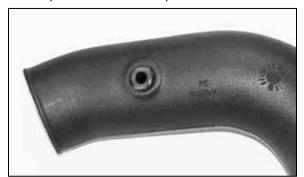
16. Install the provided grommet into the  $K\&N^{\otimes}$  intake tube as shown.
