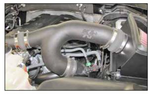
19. Install the K&N® intake tube into to turbo inlet hoses and then into the hose at the throttle body, adjust the tube for best fit and then secure with the provided hose clamps.
