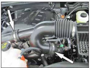
6. Loosen the hose clamps securing the intake tube the two turbo inlet tubes and then remove the intake tube from the vehicle.
