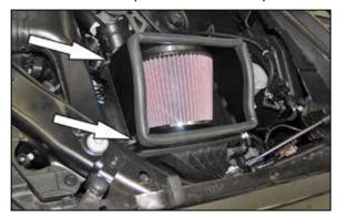
12. Install the heat shield/filter assembly onto the loser air filter housing and secure with the factory retaining clips.
