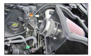
13. Install the provided coupling hose (08699) onto the filter adapter and secure with the provided hose clamp.
