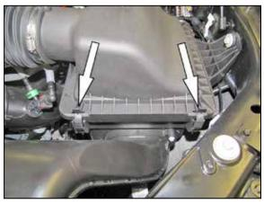
Release the two clips securing the upper air filter housing.
