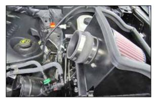
13. Install the provided coupling hose (08699) onto the filter adapter and secure with the provided hose clamp.
