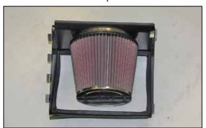
11. Install the K&N® air filter onto the filter adapter and secure with the provided hose clamp.
