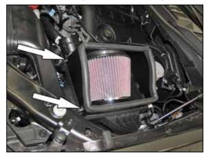
12. Install the heat shield/filter assembly onto the lower air filter housing and secure with the factory retaining clips.
