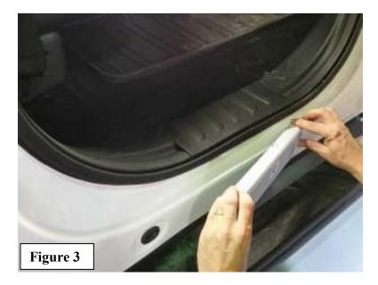
6. Press door sill to the vehicle matching the radius of the door sill with the radius of the vehicle. Hold in position for 30 seconds to ensure proper adhesion. Remove protective film. See Figure 4 for proper alignment.
