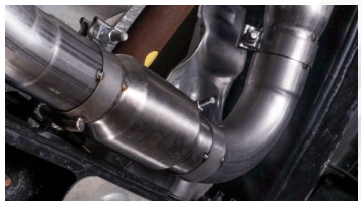
Header Leads Close-up
