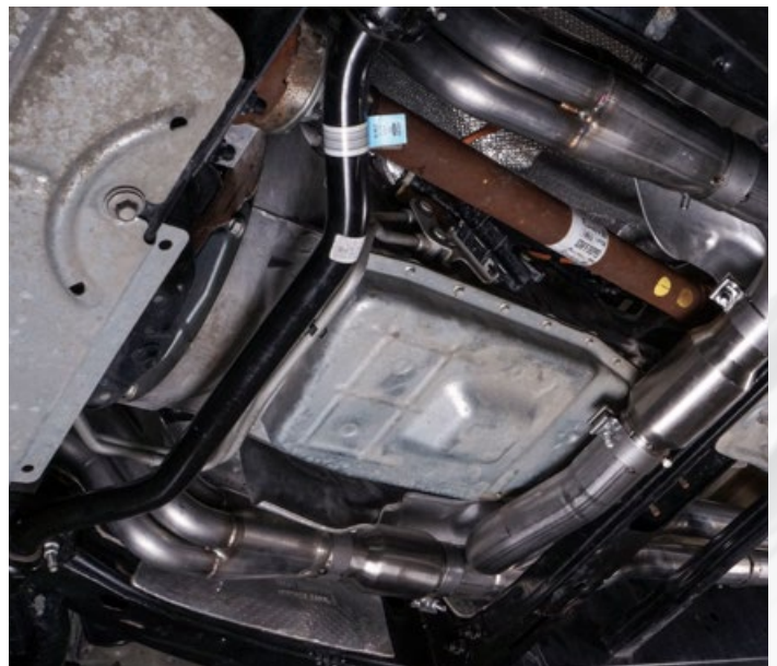
Installed Headers Close-Up
