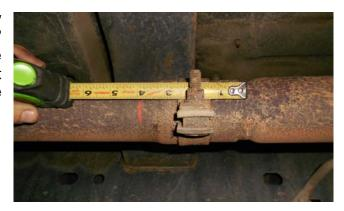
4) Now you can slide the muffler/tailpipe assembly to the rear to disengage the rubber hanger mounts that support it. Once free, the assembly can be removed by working it forward over the rear axle. (If you are working on the ground it may be easier to cut the tailpipe off at the rear of the muffler to simplify removal.)
