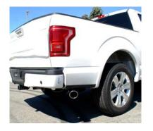
MAKE SURE YOU HAVE A 1" CLEARANCE ON ALL RUBBER BRAKE LINES, SHOCK BOOTS, TIRES, FUEL LINES, ETC..
