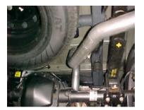
INSTALL OVERAXLE TAILPIPE #C INTO MUFFLER 1 ½" TO 2". INSERT HANGERS INTO RUBBER GROMMETS.USE CLAMP #E TO SECURE PIPE TO MUFFLER.DO NOT TIGHTEN.
