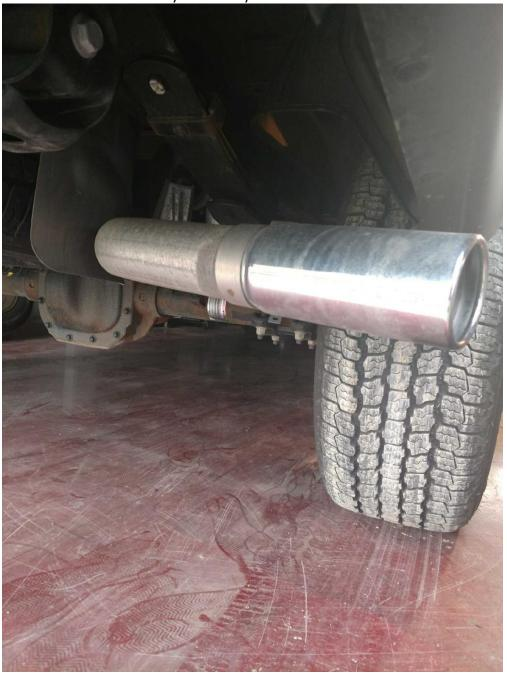
o If you factory exhaust system has a significant amount of rust, spay the bolts/nuts with penetrating oil prior to starting the work. Also spray the rubber exhaust hangers to help in removal later.
