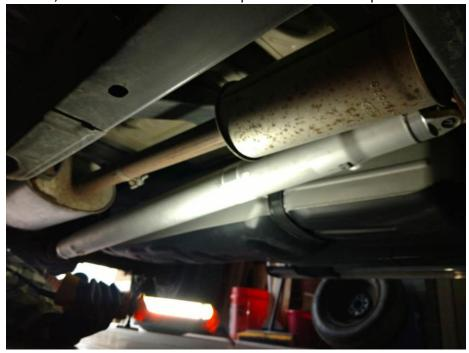
• At the front of the head pipe is a flange where it meets the factory y-pipe. Using a 13mm socket or wrench, remove the bolts from the flange.
