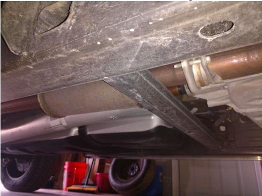
While not required, removing the exhaust hanger in front of the muffler aids in removal of the factory exhaust system. To remove the hanger from the frame,
