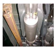
INSTALL MUFFLER # B ONTO HEADPIPE 1 ½" TO 2". USE CLAMP # G TO SECURE MUFFLER TO HEADPIPE. DO NOT TIGHTEN. USE A JACK STAND TO HOLD UP THE MUFFLER. OUTLETS SHOULD BE LEVEL.
