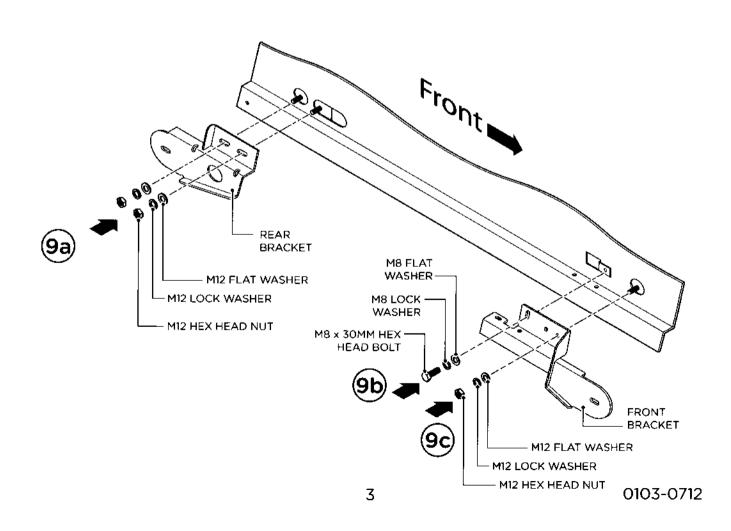
10. Fasten the bottom of the Front Bracket to the Pinch Weld of the Rocker Panel using two (2) M8 X 30 Hex Head Bolts, four (4) M8 Lock Washers, four (4) M8 Flat Washers and two (2) M8 Hex Head Nuts.
