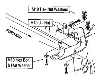
Figure 1. Driver Side - Front Bracket
