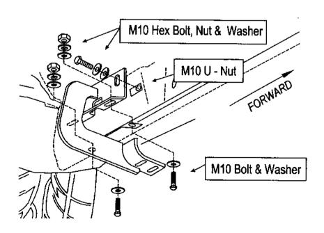
Figure 2. Driver Side - Rear Bracket
