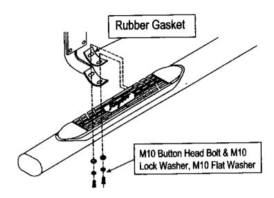
Figure 3. Installation View of Bracket & Bar
