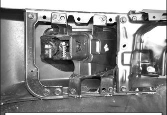
(Fig 1) Remove fog light assembly from bumper
