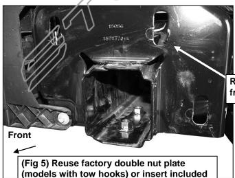
**Double Nut Plate into end of frame**
