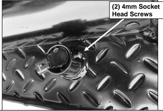
(Fig 8) Remove plugs from holes in bumper. Insert sensor (if equipped) into socket on back of bumper.
