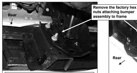
(Fig 3) Remove the factory hex nuts attaching bumper assembly to frame. STD tow package model pictured (no receiver hitch)
