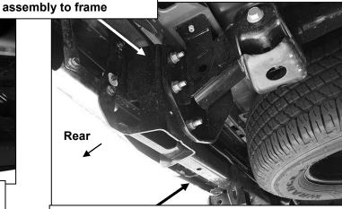
(Fig 4) Note bumper with integrated receiver hitch. Hitch cannot be reinstalled with Elevation Bumper
