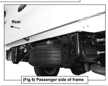
WARNING! To avoid injury or damage to the vehicle, do not remove bumper bolts unless the bumper is properly supported on blocks and/or stands or the bumper may fall.
