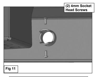
**IMPORTANT**: Sensors fit snug in sockets. The 4mm Screws are used to apply slight pressure to lock the sensors in place. Tighten both screws evenly until they touch the sensor body only. Do not overtighten screws or damage to sensors will result
