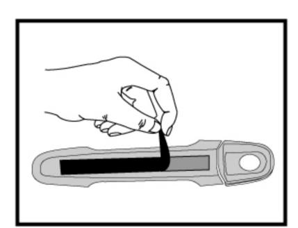
Step 3: Peel off the adhesive tape from the door handle and gently position the insert on the original equipment part and press it firmly.
