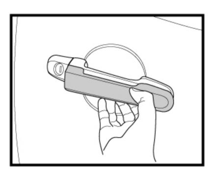
Step 2: Accurately measure the door handle position prior application. Repositioning of the double-sided tape can deteriorate their adhesive property.
