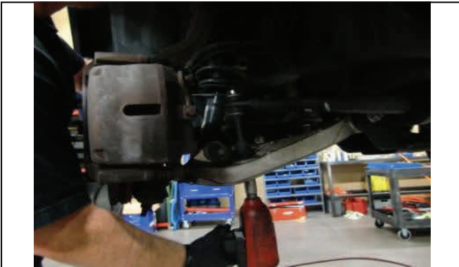
Remove lower sway bar endlink hardware.
