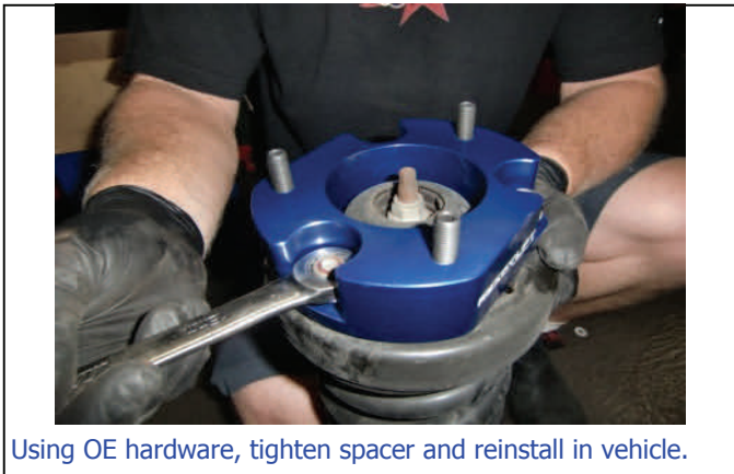
Apply thread locker to the studs and tighten in spacer
