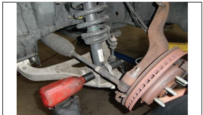
Loosen lower strut bolt/nut and remove.
