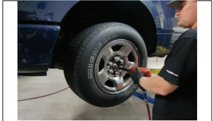
Lift vehicle securely and remove wheels/tires.
