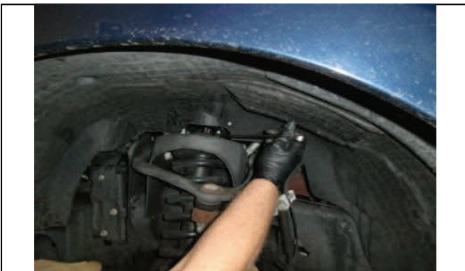
Loosen upper strut mount nuts.
