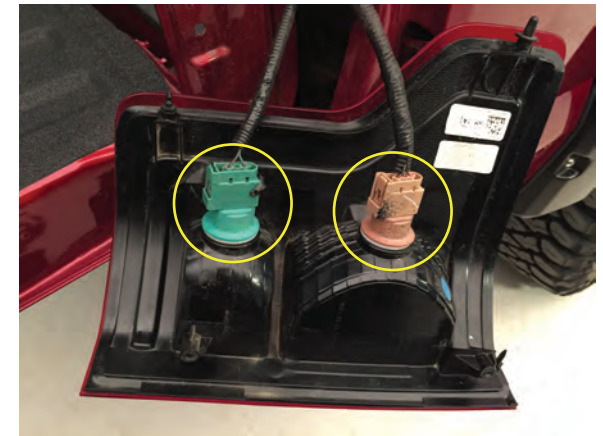
Step 3 Disconnect the factory plugs from the stock tail light.
