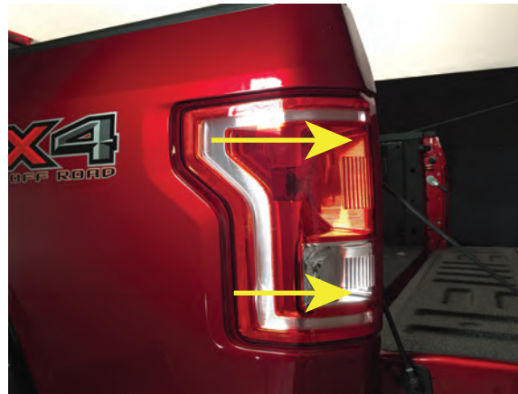
Step 2 Remove the tail light by applying firm pressure rearward.
