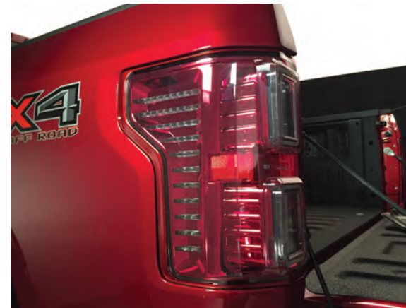
Step 5 Re-install the new tail lights in reverse order.
