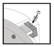
Install the supplied locknuts onto the threaded studs to secure clip to bridge. Tighten with 3/8-inch wrench or socket to 25 inch pounds. Over tightening could pull stud through aluminum bridge.
