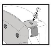
Install the supplied locknuts onto the threaded studs to secure bridge to clip. Tighten with 3/8-inch wrench or socket to 25 inch-pounds. Over tightening could pull stud through aluminum bridge.
