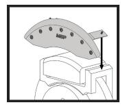
Place the caliper cover on the brake caliper. Cover should be centered across the front. Caliper cover bridges should be positioned against the brake caliper bracket.
