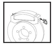
Slide the stainless steel clips on each side of the brake caliper bracket. Fit should be snug and secure.
