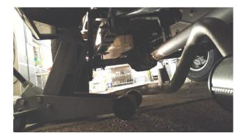
4. At this point the stock exhaust should be fully disconnected, dropped and resting on the rear axle. Simply pull the stock exhaust over the rear axle towards the front of the truck to complete the removal.
