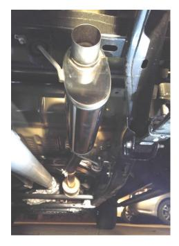
3. Now install the new over the axle pipe by using the supplied band clamp on the muffler.
