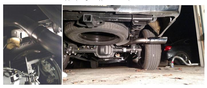
4. Lastly, reinstall the remaining factory muffler hanger and connect the final pipe. This piece will require you to connect back to the over the axle pipe, couple the connection, and ensure the exhaust tip is in the desired position.
