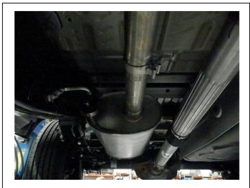
**Step 1.** To remove the OEM exhaust system, loosen the clamp attaching the systems inlet pipe to the resonator outlet pipe. Disengage all welded hangers from the OEM rubber insulators. Do not discard the OEM clamp or damage the rubber insulators as they will be needed to mount your new MAGNAFLOW system.
