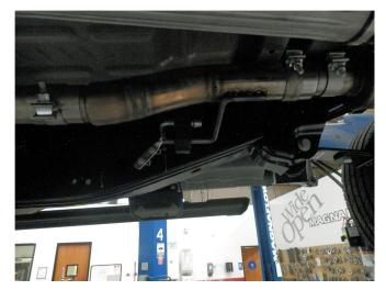
**Step 2.** Install the new system by attaching the Inlet Pipe Assembly to the resonator outlet pipe using the existing clamp. Locate the welded hanger to the rubber insulator. Leave all clamps and fasteners loose for final adjustment of the complete system once installed.
