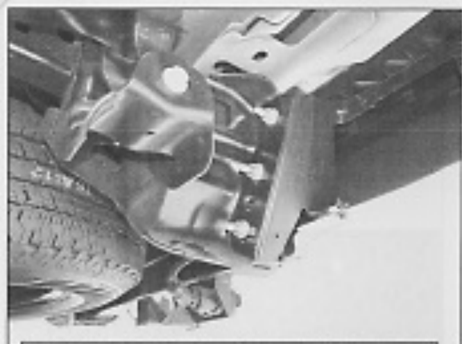
(Fig 3) Remove (3) hex nuts per side to remove bumper reinforcement or receiver hitch
