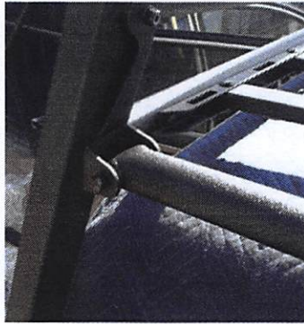
Figure 27: The cross tube mounted to the riser assembly
