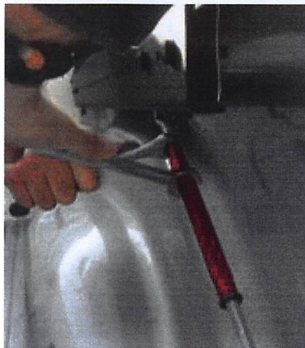
Figure 16: The jam nuts securing the turnbuckle
