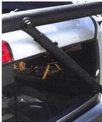
Figure 28: The headache tube secured to the cross tube
