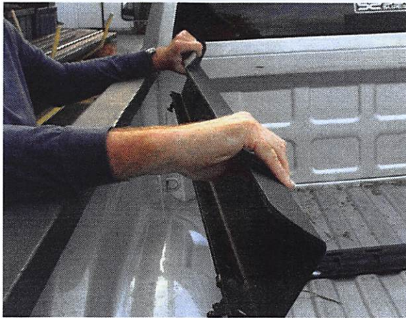
Figure 6: The bed rail being test fit onto the vehicle.
