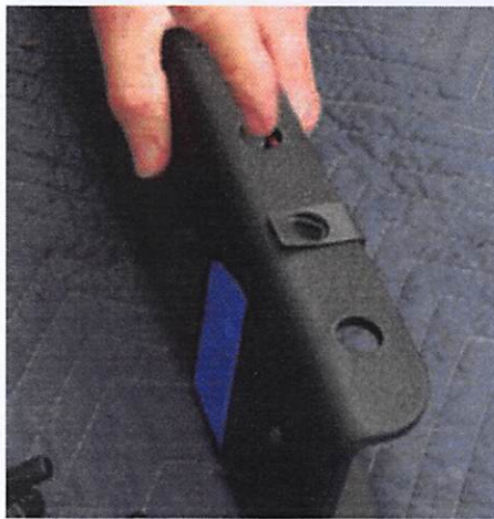
Figure 10: The clip nut installed onto the bed rail.
