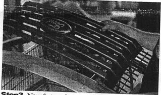
**Step3.** Now that you have completed cutting the center portion of the grille you will now be able to remove the center of the stock grille shell.
