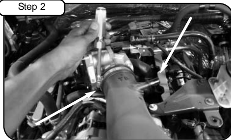
Step 2 With 5/16" nut driver loosen clamp at throttle body. Disconnect and remove OE crank case line.
