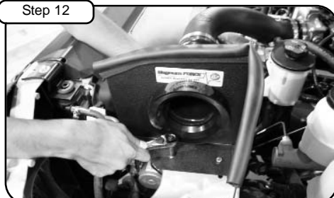
Step 12 Tighten housing using 11mm socket or wrench. Install 3/4" trim seal to housing.
