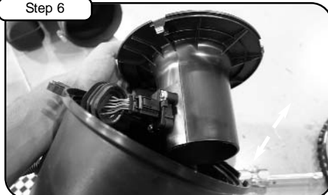
Step 6 Disconnect band clamp and with flat head screwdriver, disconnect other end of MAF harness. Carefully pull out OE MAF sensor tube.
