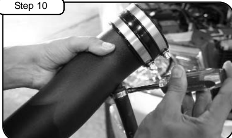
Step 10 Place 5/8" hose to new tube with mini clamp provided and tighten using 1/4" nut driver. Install couplers with clamps provided to new tube.
