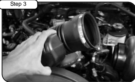
Step 3 Loosen the clamp at air box side and remove OE intake tube.
