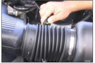
1.Disconnect The Negative Battery Terminal! Disconnect valve cover breather hose from factory intake tube and valve cover.
