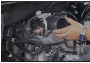
**6.** Install supplied silicone reducer on end of throttle body. Install #48 hose clamp on small end of the reducer and #56 hose clamp on the big end of the reducer. Leave hose clamps loose until final assembly.
