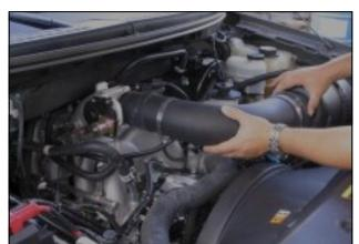
7. Install the Airaid Modular Intake Tube on engine.
